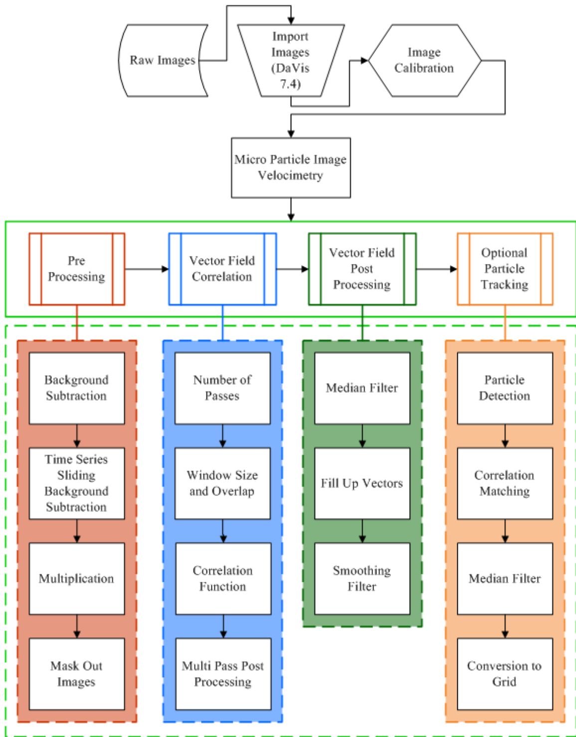
Figure 4.21: A flow chart of the sequence of image processing operations for micro particle image velocimetry..
