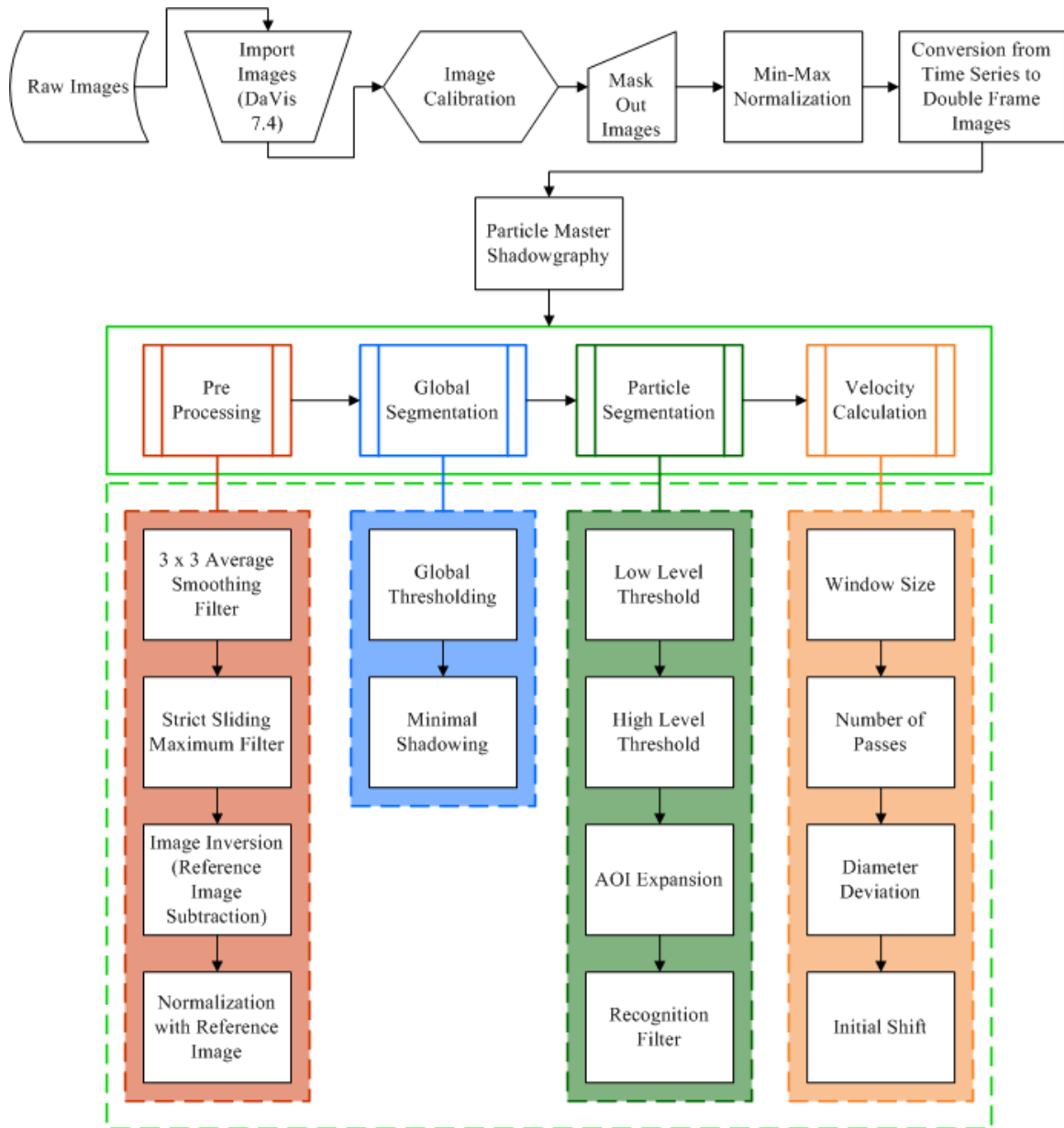
Figure 4.19: A flow chart of the sequence of image processing operations for Photobleaching MTV.
